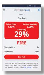
Press Start Test to perform a fire test, this works by running a test algorithm to lower the output power, the receiver sees this as obscuration.
